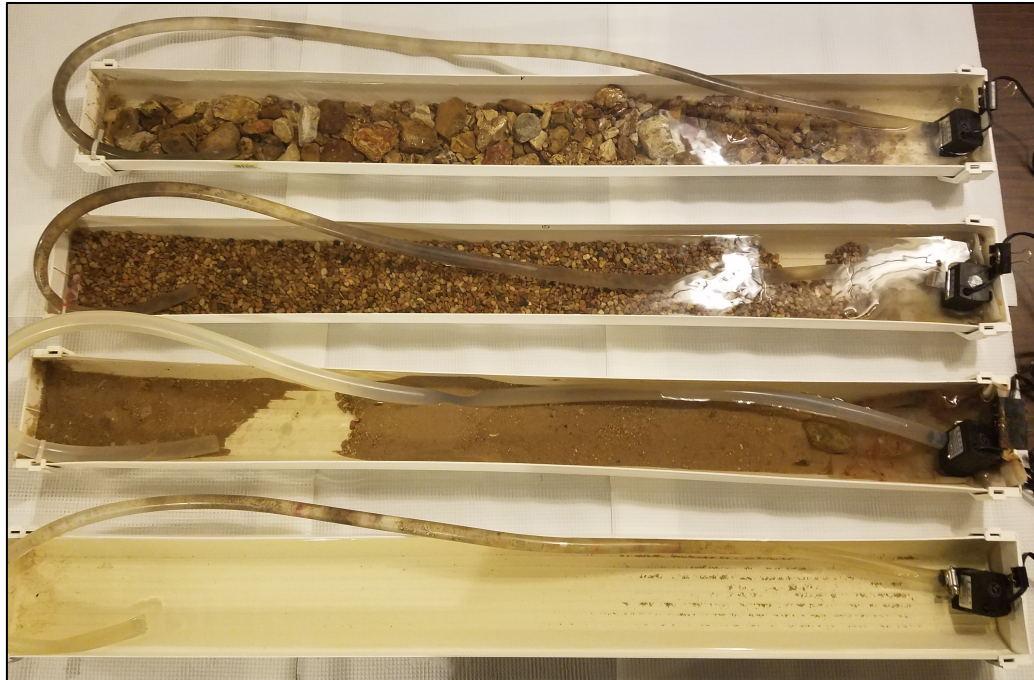
Figure 3.3. Sedimentation and adsorption experimental setup. Four gutter mesocosms with different sediment bottoms were used as treatments in this experiment. From top to bottom: (1) Mill Creek stream substrate, (2) aquarium gravel, (3) sand, and (4) control (no sediment).
